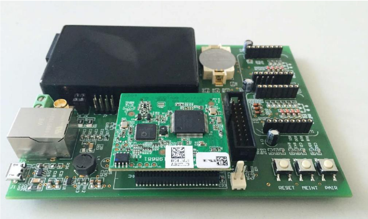
Fig 2: Picture of the devolo Green PHY eval board II (side view)
